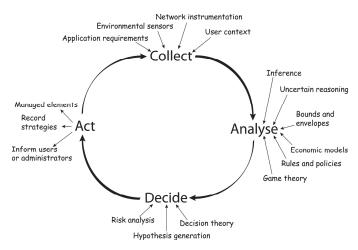
Figure 1 Autonomic control loop [23].
