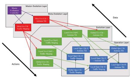
Figure 4 Example controller hierarchy split by layer.
